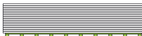
Ensure boards are on a flat surface or bearers max. 400mm apart
